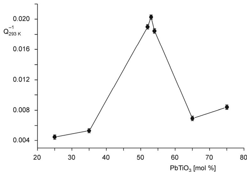
Fig. 1. Dependences of the internal friction background on the PbTiO<sub>3</sub> concentration in PZT ceramics obtained via the synthesis by the sol-gel method
