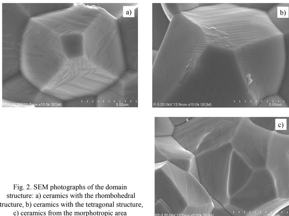
Fig. 2. SEM photographs of the domain structure: a) ceramics with the rhombohedral structure, b) ceramics with the tetragonal structure, c) ceramics from the morphotropic area
